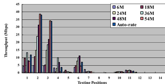
Figure 4: Measured throughputs at different positions when data rate is set to 6 Mbps, 18 Mbps, 24 Mbps, 36 Mbps, 54 Mbps and auto rate respectively
