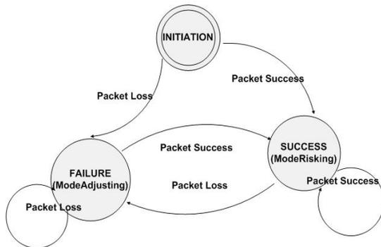
Figure 5: State transition diagram of CORA
