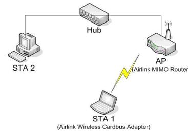
Figure 2: NIC testing network topology
