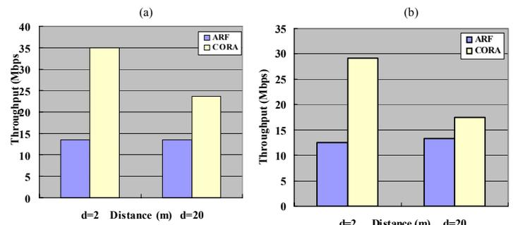
Figure 10: Collision scenario (a): with packet size from 1000 to 1400bytes (b): with packet size from 400 to 1400bytes
