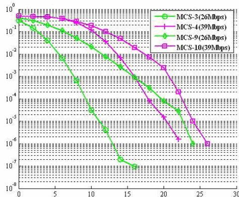
Figure 1: SNR-BER Curves of MCS 3, 4, 9, 10 under Rayleigh channel. Data rates of MCS 3 and 9 are both 26 Mbps. MCS 4 and 10 both mirror 39 Mbps.
