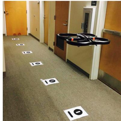
**Figure 1: DroneSense in action, collecting Wi-Fi signals in a hallway using its built-in Wi-Fi radio. Paper marks on the floor indicate the target measurement locations.**
