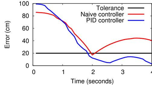
**Figure 4: Comparing a naive controller with the PID controller by flying the drone to a target location from 1 meter away. The PID controller successfully reaches the target faster while the naive controller suffers from overshooting.**
