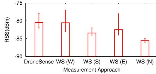
**Figure 5: Comparing the signal measurements of DroneSense and the walking sense (WS) approach at a given measurement location. By involving human interactions in the measurement collection, the measurements from WS are affected by the human body.**
