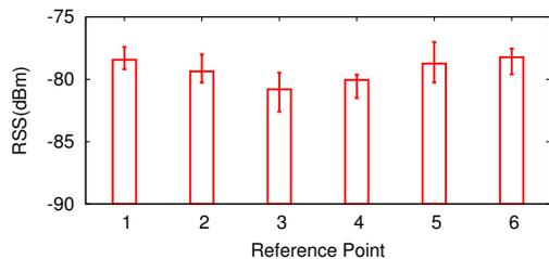
**Figure 6: Repeating wireless measurements by DroneSense along a flight path of 6 reference points for 10 times. The measurement variation for a location is around 2dB and no more than 3dB. We conclude that DroneSense is accurate enough for wireless measurement.**
