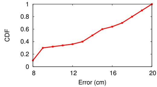
**Figure 3: Navigation Error CDF. The mean error is 13 centimeters, and the max error is 20 centimeters.**
