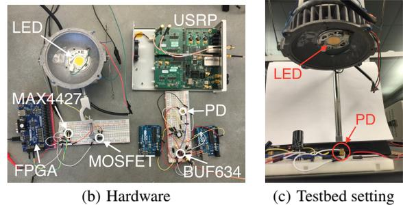
**Figure 2: DarkVLC implementation.** The LED is driven by a Xilinx Artix-7 FPGA through a MOSFET (STF5N52U) and a gate driver (MAX4427). The photocurrent generated by the photodiode is converted to the voltage signal by a resistor. The voltage signal is sampled by a USRP with an LFRX daughterboard. The voltage follower (BUF634) between the resistor and the USRP is for impedance matching.
