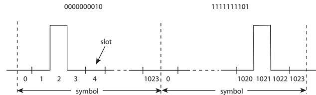
**Figure 1: Pulse Position Modulation (PPM).** A light pulse occurs only once per symbol. Each symbol is divided into 1024 time slots, thus the time slot where the light pulse resides represents 10-bit information.
