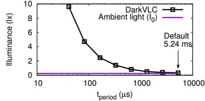
**Figure 4: DarkVLC luminance w/ varying  $t_{\text{period}}$ .**
