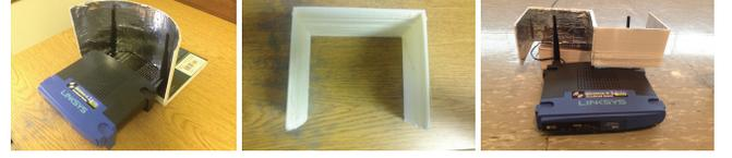
(a) Concave reflector (b) Partial square-wave reflector (c) Square-wave reflector with a metal layer
