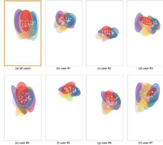
Figure 3: Imaginary keyboard positions and the inferred key distributions (95% confidence ellipses) for back-of-device word-gesture input. The borders illustrate the boundaries of the back screen of the smartphone. (a): the average distribution of all participants. (b) to (h): key distributions obtained from 7 participants randomly picked from all participants.
