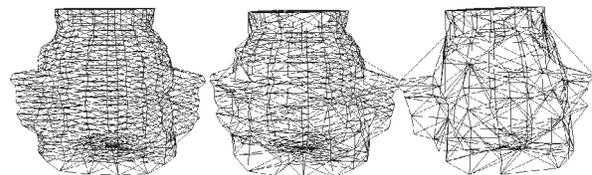
**Figure 1:** The mesh of a nutcracker toy model at various levels-of-detail, with (left) 1260, (middle) 950 and (right) 538 triangles respectively.
