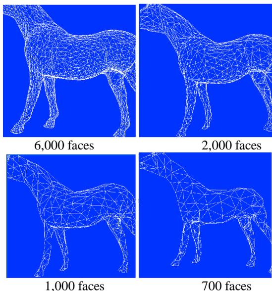
**Figure 8:** A horse mesh with original resolution of 6,000 faces, and three other levels-of-detail generated by the PM algorithm.
