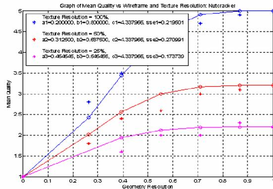
**Figure 6:** Pan et al. [19] showed in perceptual experiments that mesh quality increases exponentially as the number of vertices increases after the minimum required resolution is reached. The visual qualities (Y-axis) of three different 3D objects were plotted against the normalized geometry resolution (X-axis).
