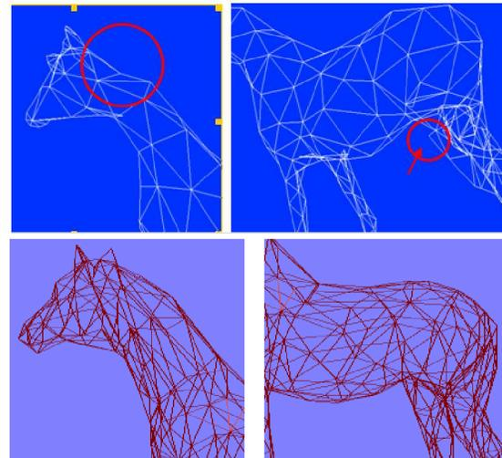
**Figure 9:** (Top) A simplified horse mesh composed of 700 faces, generated by the PM algorithm, shows noticeable degradation of visual quality. (Bottom) Corresponding mesh surface generated by the QEM algorithm shows smoother silhouettes.
