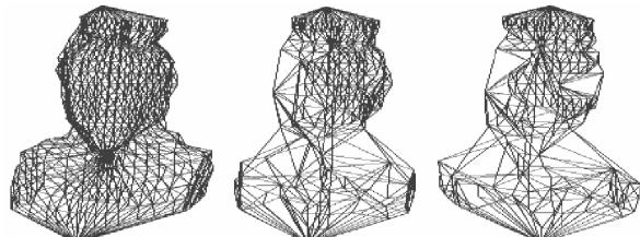
**Figure 7:** The left mesh (1,296 faces) is the original. Both the middle (614 faces) and the right mesh (502 faces) are of unsatisfactory visual
