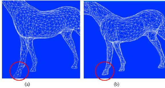
**Figure 10:** A simplified horse mesh composed of 3,000 faces generated by the PM (a) and QEM (b) algorithm.
