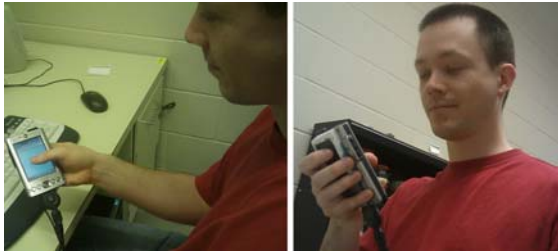
Figure 1 In the experiment, we asked participants to sit in a chair, and perform the target selection task using one hand. The touchpad on the back is operated using the index finger.
