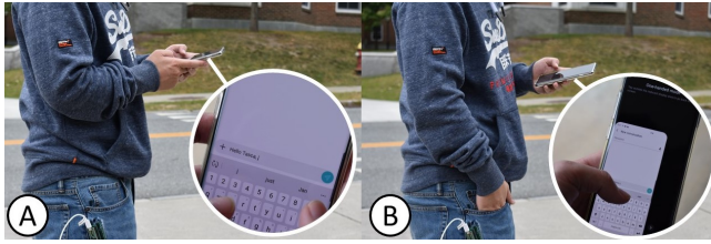
Figure 8: Our system can sense user activity by tracking if a user puts their hands in the pocket. (A) When typing using both hands, the keyboard is configured in its maximum width. (B) The system detects that the user puts their hand in the pocket. (C) The system automatically switch the keyboard to a narrower version to facilitate typing using one hand.
